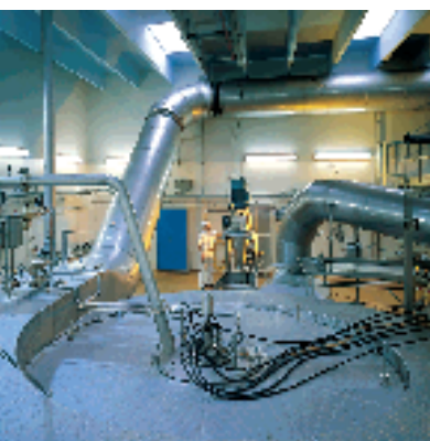
Dryer operating with either nozzle or rotary atomizer
